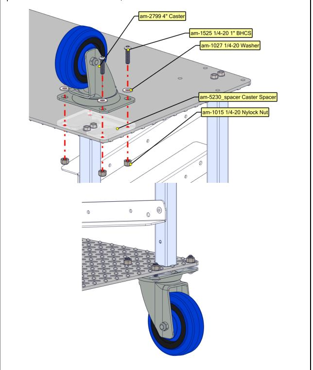
Step 7 Repeat Step 5 with the three remaining Casters. Ensure the remaining Caster without a brake is placed on the side with the raised end of the shelving. am-4989 Caster with Brake am-4989 Caster with Brake am-2799 Caster am-2799 Caster
